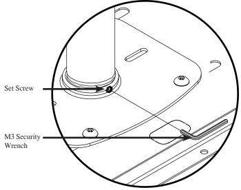
**Step 4.** Use an M3 security wrench to tighten the set screw.
